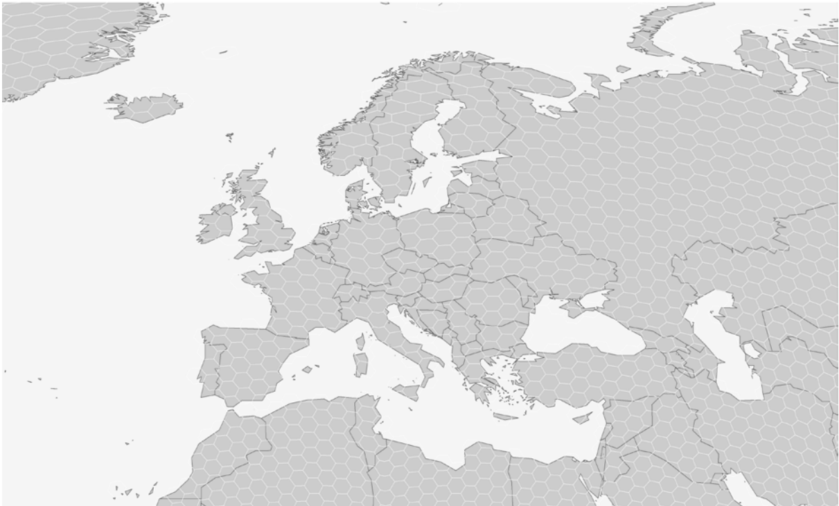
Figure 1: Level 8 Icosahedral Snyder Equal Area Aperture 3 Hexagon Discrete Global Grid
